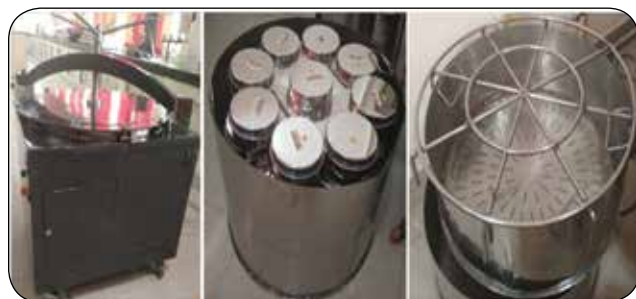
Fig: (a) Hawaijar maker (b) Fermenting Unit (c) Soaking and Cooking Unit
