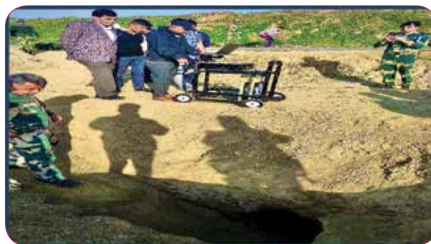
Fig 1: Radio Frequency Device for Detection, Imaging and Mapping of Underground Utilities
