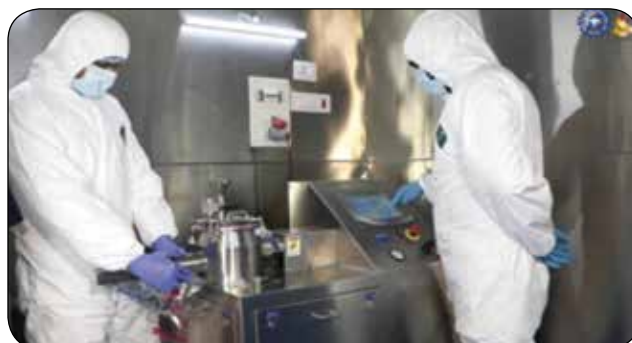
Rapid Mixer Granulator with 3Kg bowl in use to prepare 1 Kg granules for tablet compression
