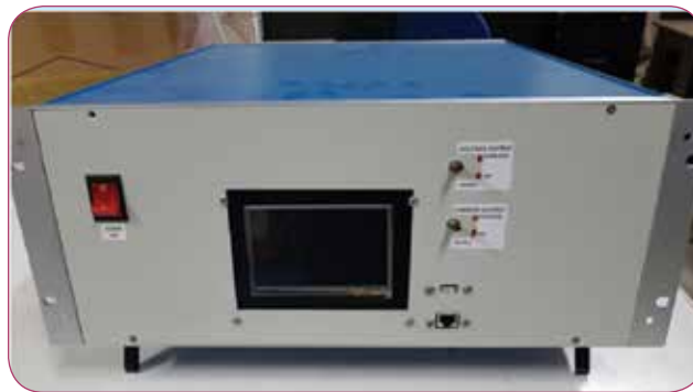
Fig:3 Prototype of 1000 Watt Calibration Grade Solid State Power Source
