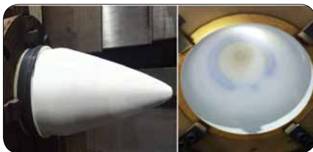
Outer profile machining in progress Inner profile machining in progress
