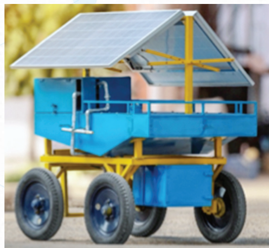
Solar operated micro irrigation applicator with drip irrigation system
