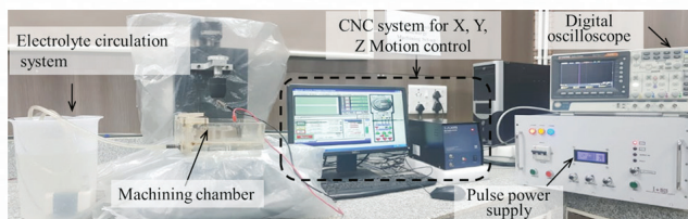
Optical image showing in-house developed 3-axis ECDM experimental set-up
