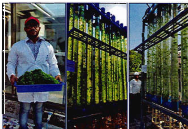
Fig. 1 Ulva Biomass harvested from 1KL Airlift tubular photobioreactor at DBT-ICT Centre for Energy Biosciences
