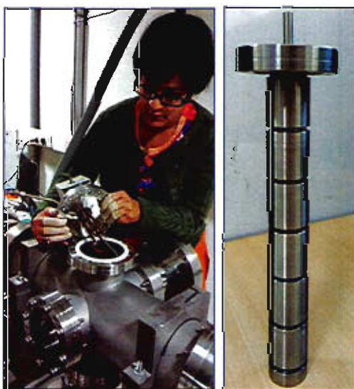
Fig. 7 Aerodynamic lens with multiple and variable size orifices
