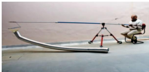
Fig 1: Final Prototype of fruit plucking device
