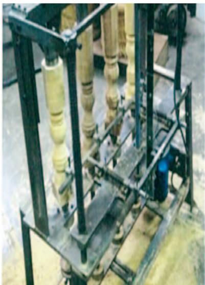
Fig 12 Final Vertical Quadripilator Lathe
