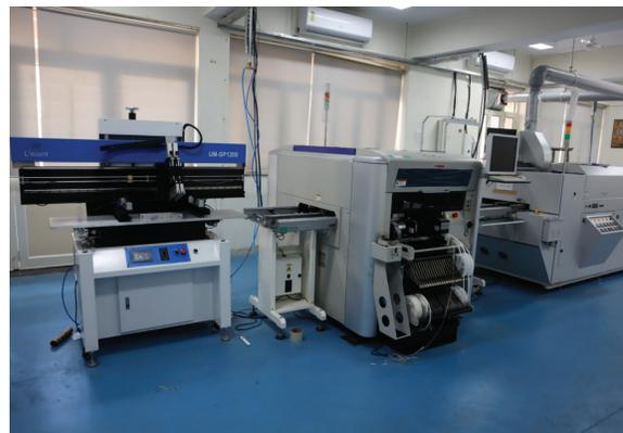
Fig 2 Surface Mount Technology (SMT) based pick and place robotic assembly unit at CRTDH Jaipur
