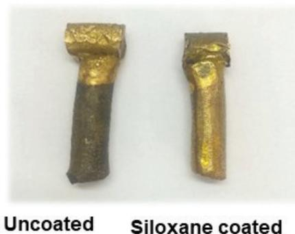
Fig 7. Siloxane coating for metal casting.
