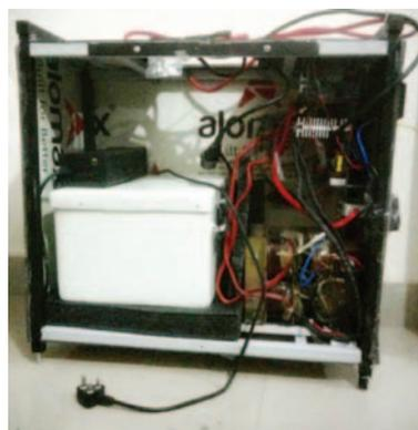
Fig 11 (b) Battery System with Charging and AC Power system
