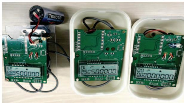
Fig 4: Final developed prototype of Static Water Meter - Aqua Management Binary Unit
