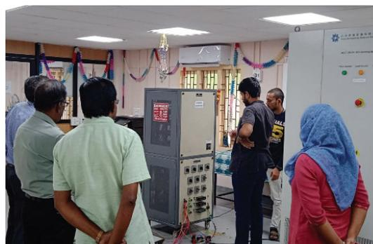
Fig 6(b): Test setup with APFC panel
