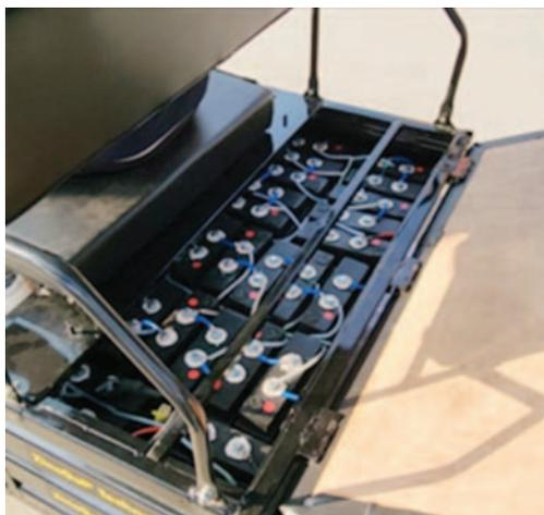
Fig. 7 (b) series of battery
