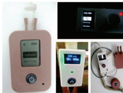
Fig. 5: Final developed prototype of Infusion Flow Monitoring Device
