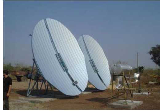
Hybrid system for solar distillation and drying application
