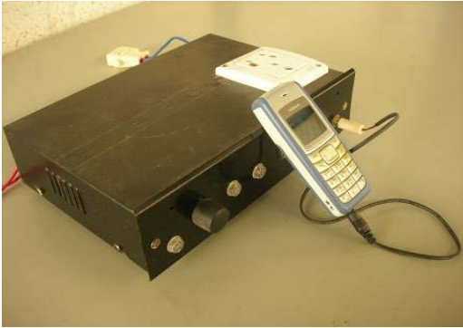
Mobile operated remote switch
