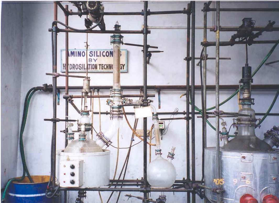
Pilot Plant for Development of Next Generation Amino Silicon Based on Hydrosilation Technology
